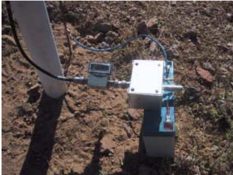
Figure 13b. Home-Made VSWR Meter Showing Excellent Source Match of Test Antenna
