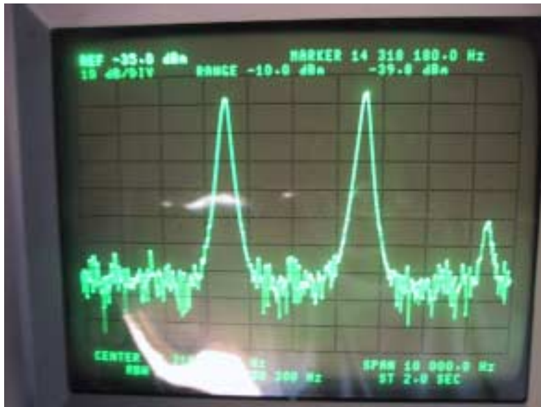
Figure 8. Representative Screen Shot of Spectrum Analyzer Used as a Calibrated Tuned Receiver
