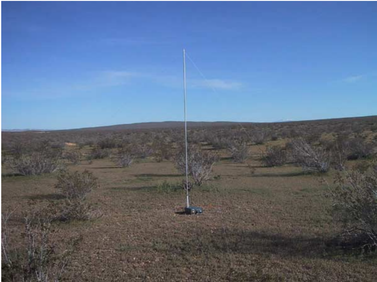
Figure 4. Reference Monopole Matched with Murch UT-2000 Transmatch
