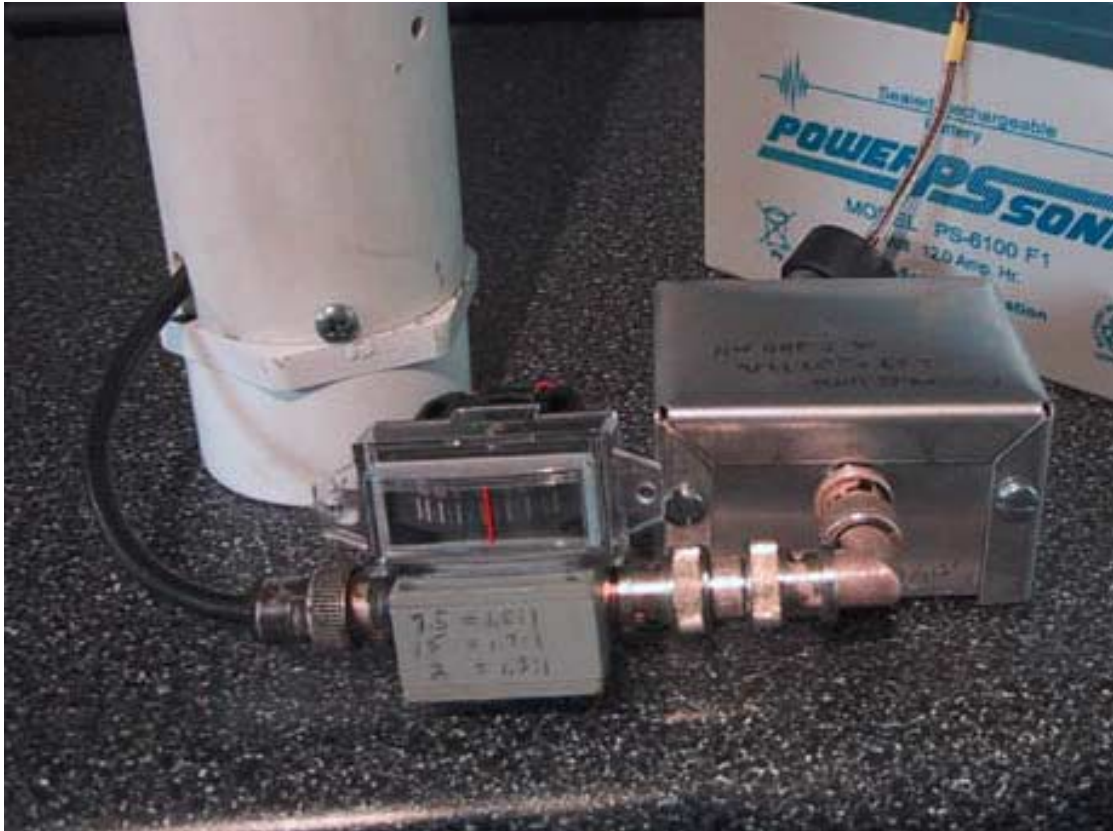
Figure 12. Small VSWR Meter Combined with Broadband Transformer
